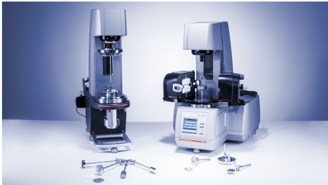
Figure 1: Modular Compact Rheometers (MCRs) equipped with a powder flow cell (left) and a powder shear cell (right).
