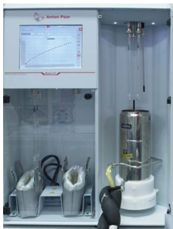
Figure 1. Recirculating Dewar and bath setup
